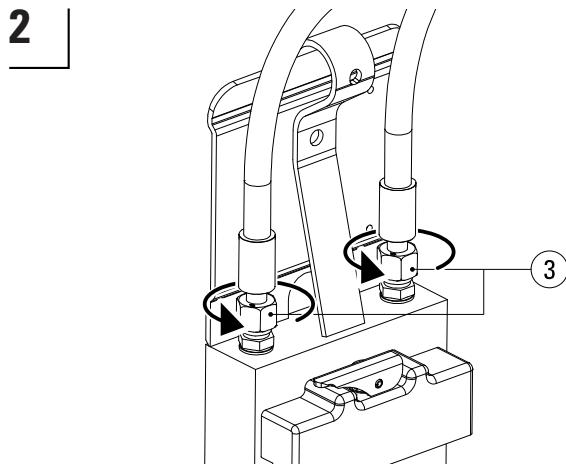
Loosen the hose connectors (3) slightly so that the pistons do not create a vacuum when removing the hydraulic parts.
