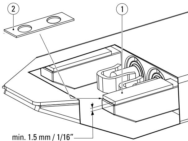
The thickness of Wear Strips (1) may not be less than 1.5 mm (1/16"). When Wear Strips (1) have worn to this thickness, replace them or fill with spacers (2) (Art. N° RE0092002). See point 3 of the Maintenance Schedule.
