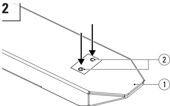
Tap the spring pins (2) out of the sleeve (1).
