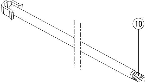
Remove remaining adhesive residue from the piston rod thread (10), then clean the piston rod and thread (10) using Loctite 7063<sup>1</sup>.
