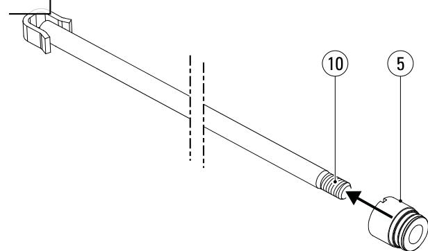
Slide the (new) cylinder head (5) onto the piston rod (10).
