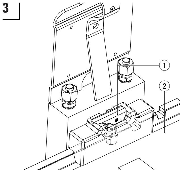
Make sure that each of the KOOI-REACHFORKS® locking pins (2) drops into one of the notches on the carriage plate. Use catch (1) before operating.
