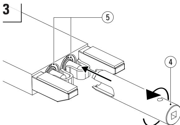
Place a drip tray below the fork. Unscrew the cylinder head(s) (5) using a cylinder head spanner (4) and a ratchet.
