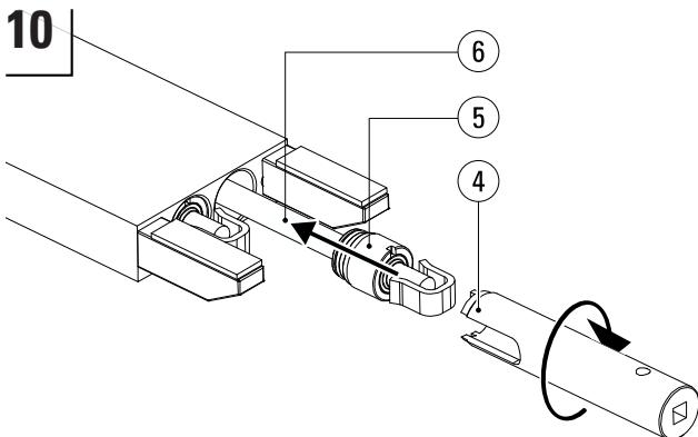
Smear Copaslip<sup>2</sup> onto the thread of the cylinder head (5). Line up the hydraulic set (6) with the cylinder and use a hammer to tap it carefully into the bore. Screw the cylinder head tight using the cylinder head spanner (4) and a torque wrench. See table below for torque values.
