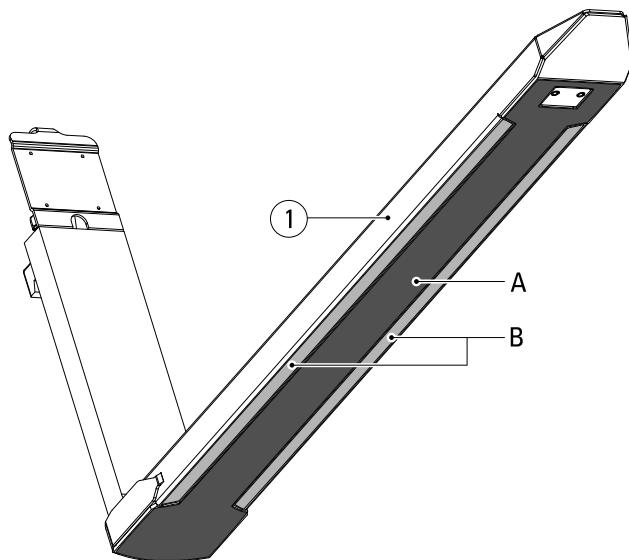
When surface A (dark grey, integrated wear plate) is worn to the extent that it is level with or below surface B (light grey), then the sleeve (1) must be replaced.
