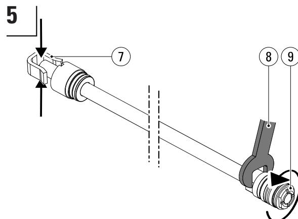
**5** Clamp the piston rod at the rod end (7), not on the piston rod itself to prevent damage (see step 4 in this chapter). Use a size 24 (8) open-ended spanner to loosen the piston (9). If the piston cannot be loosened, heat the piston with a burner.
