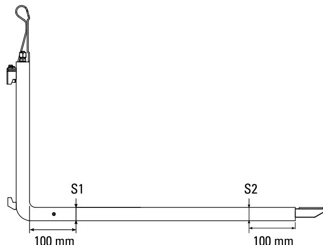
The inner fork must be replaced when S1 is 5% thinner than S2. See point 7 of the Maintenance Schedule.
