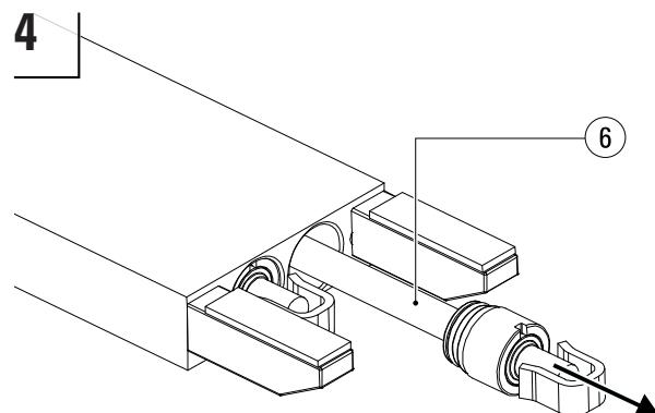
**4** Pull the entire hydraulics set (6) consisting of the piston, cylinder head and piston rod out of the fork.
