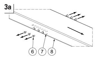
Applies only to: KOOI-REACHFORKS® type TRG2; Unscrew the screws (6) (on both sides) from the stops (7) and remove the inner sleeve. **Tools required:** Allen key 4.
