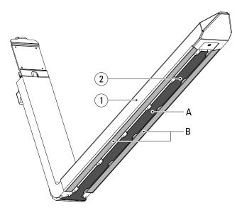
Applies only to: KOOI-REACHFORKS® type RGE and RGEN; When surface A (dark grey, integrated wear plate) is worn to the extent that it is level with or below surface B (light grey), then the sleeve (2) must be replaced. If there are signs of wear in the lower side of the sleeve (2) then it must be replaced. See point 4 of the Maintenance Schedule.
