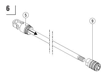
When piston (9) is removed, the cylinder head (5) can be removed, should it need to be replaced.
