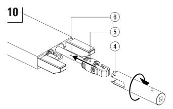
Smear Copaslip<sup>2</sup> onto the thread of the cylinder head (5). Line up the hydraulic set (6) with the cylinder and use a hammer to tap it carefully into the bore. Screw the cylinder head tight using the cylinder head spanner (4) and a torque wrench. See table below for torque values. **Tools required**: Hammer, Copaslip<sup>2</sup>, cylinder head spanner\*, 1/2" ratchet.
