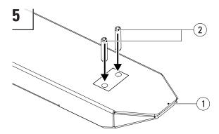
Tap the spring pin(s) (2) into the (new) sleeve (1).
