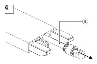
Pull the entire hydraulics set (6) consisting of the piston, cylinder head and piston rod out of the fork.
