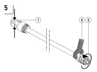
Clamp the piston rod at the rod end (7), not on the piston rod itself to prevent damage (see step 4 in this chapter). Use a size 24 (8) open-ended spanner to loosen the piston (9). If the piston cannot be loosened, heat the piston with a burner.
