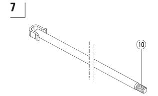
Remove remaining adhesive residue from the piston rod thread (10), then clean the piston rod and thread (10) using Loctite 7063<sup>1</sup>.
