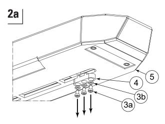
Applies only to: KOOI-REACHFORKS® type TRG2; Unscrew the screws (3a + 3b) and remove the stops (4) from the outer sleeve (5) (on both sides of the sleeve). **Tools required:** Allen key 4.
