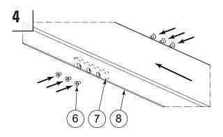
Applies only to: KOOI-REACHFORKS® type TRG2; Slide the (new) inner sleeve (8) onto the fork. Tighten the screws (6) (on both sides in the stops (7). Lock the screws (6) with Loctite 270<sup>1</sup>.
