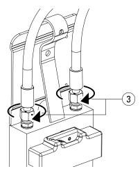
Screw the hose connectors (3) tight. **Tools required**: Open-ended spanner 22.
