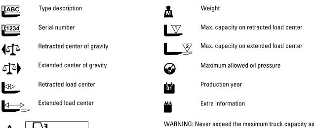
WARNING: Never exceed the maximum truck capacity as seen on the truck type plate. Rated capacity of both truck and attachment is the responsability of the original truck manufacturer and may be less then the capacity shown on the attachments type plate.
