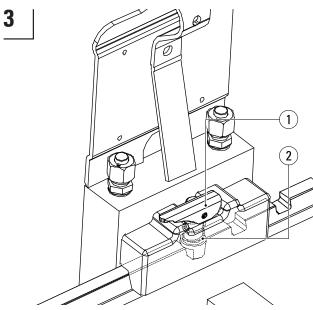
Make sure that each of the KOOI-REACHFORK® locking pins (2) drops into one of the notches on the carriage plate. Use catch (1) before operating.
