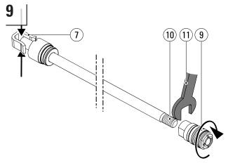
Apply Loctite 270 to the thread (10) of the piston rod <sup>1</sup>. Clamp the piston rod at the rod end (7), not on the piston rod itself to prevent damage (see step 4 in this chapter). Clean the piston thread with Loctite 7063<sup>1</sup>. Use a torque wrench 24 (11) to tighten the piston (9) onto the piston rod (10) to a torque of 100 Nm.
