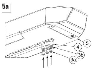
Applies only to: KOOI-REACHFORKS® type TRG2; Place the stops (4) in the outer sleeve (5). Tighten the screws (3a + 3b) (on both sides of the sleeve). Lock the screws (3) with Loctite 270<sup>1</sup>. **Tools required:** Allen key 4, Loctite 270<sup>1</sup>.
