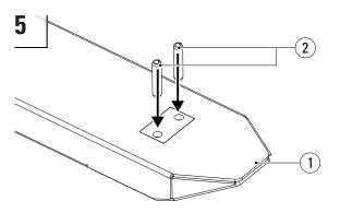
Tap the spring pin(s) (2) into the (new) sleeve (1).
