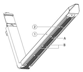
Applies only to: KOOI-REACHFORKS® type REE and REEN; When surface A (dark grey, integrated wear plate) is worn to the extent that it is level with or below surface B (light grey), then the sleeve (2) must be replaced. If there are signs of wear in the lower side of the sleeve (2) then it must be replaced. See point 4 of the Maintenance Schedule.
