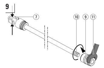
Apply Loctite 270 to the thread (10) of the piston rod <sup>1</sup>. Clamp the piston rod at the rod end (7), not on the piston rod itself to prevent damage (see step 4 in this chapter). Clean the piston thread with Loctite 7063<sup>1</sup>. Use a torque wrench 19 or 24 (11) to tighten the piston (9) onto the piston rod (10) to a torque of 70 Nm.
