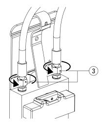
Loosen the hose connectors (3) slightly so that the pistons do not create a vacuum when removing the hydraulic parts.
