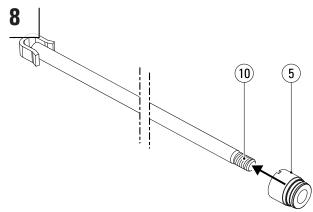
Slide the (new) cylinder head (5) onto the piston rod (10).
