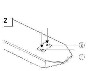
Tap the spring pins (2) out of the sleeve (1). **Tools required**: Hammer, punch Ø10
