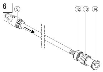
When the piston section 1 (14) has been removed the piston seal (13) can be replaced if necessary. When piston section 2 (12) is also removed, the cylinder head (5) can be removed, should it need to be replaced.
