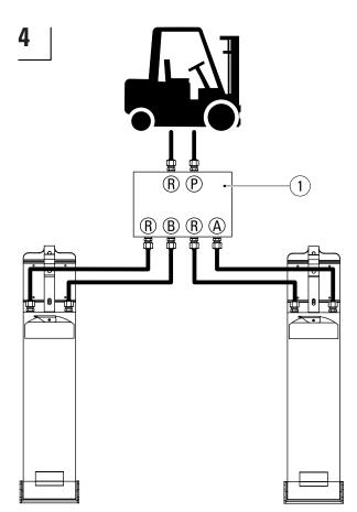
Connect the KOOI-REACHFORKS® to the hydraulic system via the flow divider (1).
