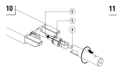
Smear Copaslip<sup>2</sup> onto the thread of the cylinder head (5). Line up the hydraulic set (6) with the cylinder and use a hammer to tap it carefully into the bore. Screw the cylinder head tight using the cylinder head spanner (4) and a torque wrench. See table below for torque values. **Tools required**: Hammer, Copaslip<sup>2</sup>, cylinder head spanner\*, 1/2" torque wrench.
