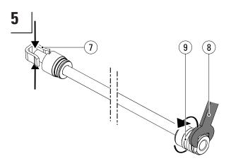
Clamp the piston rod at the rod end (7), not on the piston rod itself to prevent damage (see step 4 in this chapter). Use a size 19 or 24 (8) open-ended spanner to loosen the piston (9). If the piston cannot be loosened, heat the piston with a burner.
