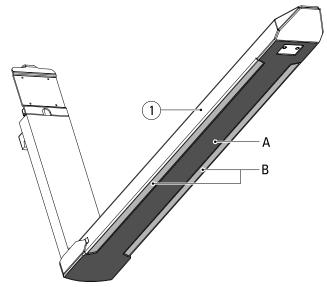
When surface A (dark grey, integrated wear plate) is worn to the extent that it is level with or below surface B (light grey), then the sleeve (1) must be replaced or fitted with a welded-on wear plate. For more information about welded-on wear plates, please contact your fork supplier. See point 4 of the Maintenance Schedule.
