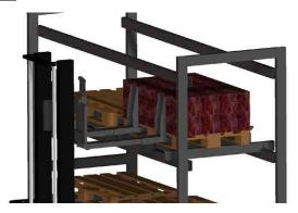
Use the forklift truck, with or without reach function, to place the forks in the pallet inserts.
