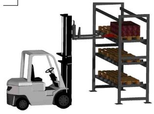
Switch on the laser and move the forks towards the pallet. Use the line laser to determine the proper height of the forks.
