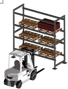
Position the forklift truck in front of the pallet as shown above.
