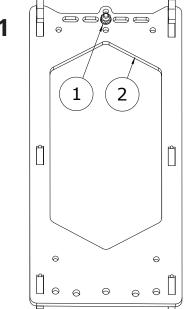
Centre the pallet bumper on the carriage plate using the positioning bolt (pos. 1).
