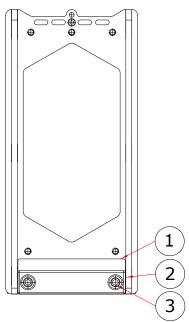
Fit the impact block (pos. 2) to the pallet bumper using the supplied bolt sets (pos. 3). NB: An extra adjusting plate (Pos. 1) is supplied for each fork shank thickness, and this can be used if the pallet still touches the base of the fork.
