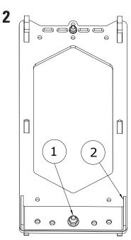
Fix the Pallet Bumper to the carriage plate by attaching the suspension bracket (pos. 2).
