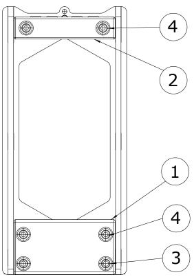
The bottom block is fixed in place at four points. The bottom two are the same as in step 3. The top two should be fixed with Loctite 243. The top block should also be fixed with Loctite 243.
